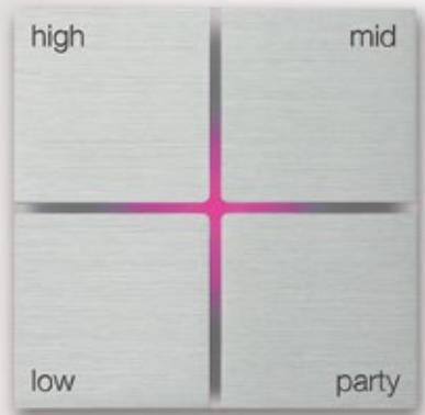
Optionally, up to four additional scenes can be launched by holding the multi-touch for a longer period, which activates the unique RGB scene sequencer.
