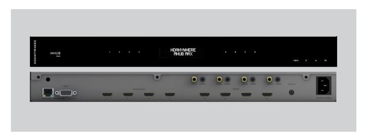
MHUB MAX is an Ultra HD Premium 4x4 HDMI 2.0 matrix with maximum bandwidth capabilities - the ultimate matrix option for cinema purists, it supports the full HDMI 2.0 (a/b) 18Gbps max data rate, capable of carrying the most premium UHD/4K 60 4:4:4 content, with all HDR formats (10 & 12-bit), Dolby Vision, HDR10+ and HLG.
