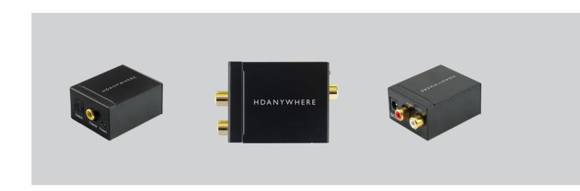
The DAC is a small and simple device that converts a digital audio input via S/PDIF optical TOSLINK or coaxial RCA connection to 2-channel analog stereo RCA L/R audio.
