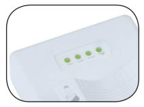
PWR: If the Power LED is On, the XAP-1240 is powered. If the Power LED is OFF, the XAP-1240 is not receiving power or the LED has been turned off in the AP's software interface. The Power LED blinks when the XAP-1240 is booting.
