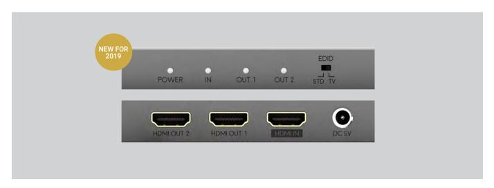
The 1x2 Splitter MAX is an Ultra HD Premium  $^{TM}$  1x2 HDMI 2.0 splitter with maximum bandwidth capabilities, the ultimate splitter option for cinema purists, it supports the full HDMI 2.0 (a/b) 18Gbps max data rate, capable of carrying the most premium UHD/4K 60 4:4:4 content, with all HDR formats (10 & 12-bit), Dolby Vision®, HDR10+ and HLG.
