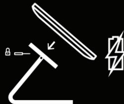
Lock Case to BaseStation if desired using lock tool.
