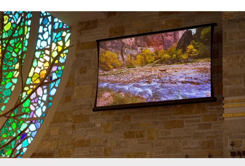
Zero-G is available with our Slate ambient-light-rejecting (ALR) screen technology which helps produce increased contrast levels and darker blacks than a white or gray screen.
