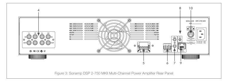
NOTE: L/R LINE IN/LOOP OUTPUT CARD CAN BE REPLACED WITH SONANCE DIGITAL INPUT MODULE (SKU 93099 SOLD SEPARATELY) FOR ULTIMATE PERFORMANCE ENHANCEMENT THROUGH DIRECT CONNECTION TO A DIGITAL SOURCE.
