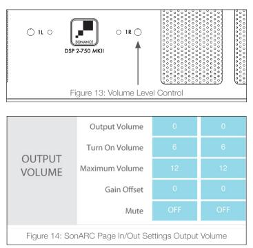
IMPORTANT: USE CAUTION WHEN SETTING VOLUME LEVELS EITHER ON THE AMPLIFIER OR AN AUDIO SWITCHER AS NOT TO OVERDRIVE AND POSSIBLY DAMAGE SPEAKERS. VERIFY ALL SOURCES AS OUTPUT VOLTAGE VARIES FROM DEVICE TO DEVICE.
