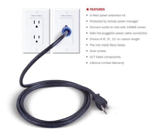
Tributaries version of the in-wall power extension kit, the PWRI-X adds a fresh take on this common idea by using the Neutrik® PowerCON® locking connector as the "inlet" plug. This gives the installer a safe and reliable connection when plugged into the wall. Plus the PowerCON® connector is physically different from other outlets making it easier to locate.
